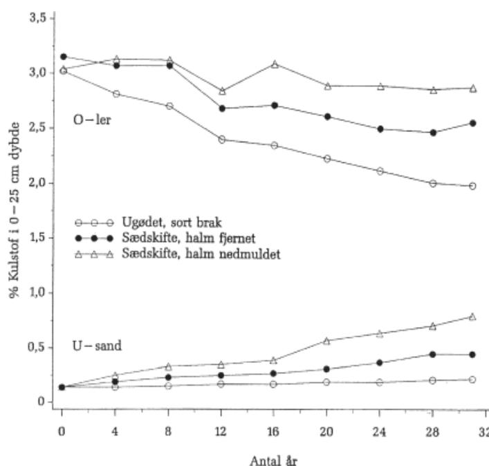
Fig.4. The content of carbon in tested fields from Aulum, Denmark, with different soil treatments over 30 years. A cautious judgement indicates that clayey soil has maximum 4% organic content and sandy soils 1% (See also Ref. 5) Compare with Annex 2.
